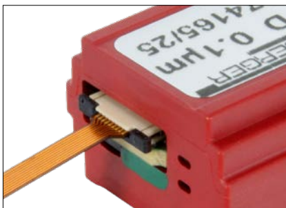
Correctly inserted sensor print
